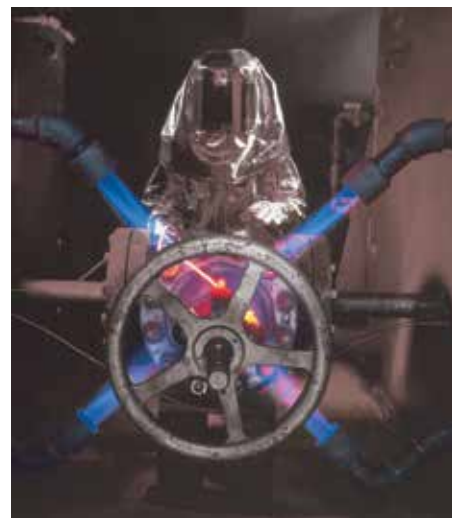
Various gasket materials including 9900, 9800, 9850 and 5500, have been tested to industry fire test standards.
